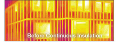
Adding exterior continuous insulation prevents heat flow through framing.
