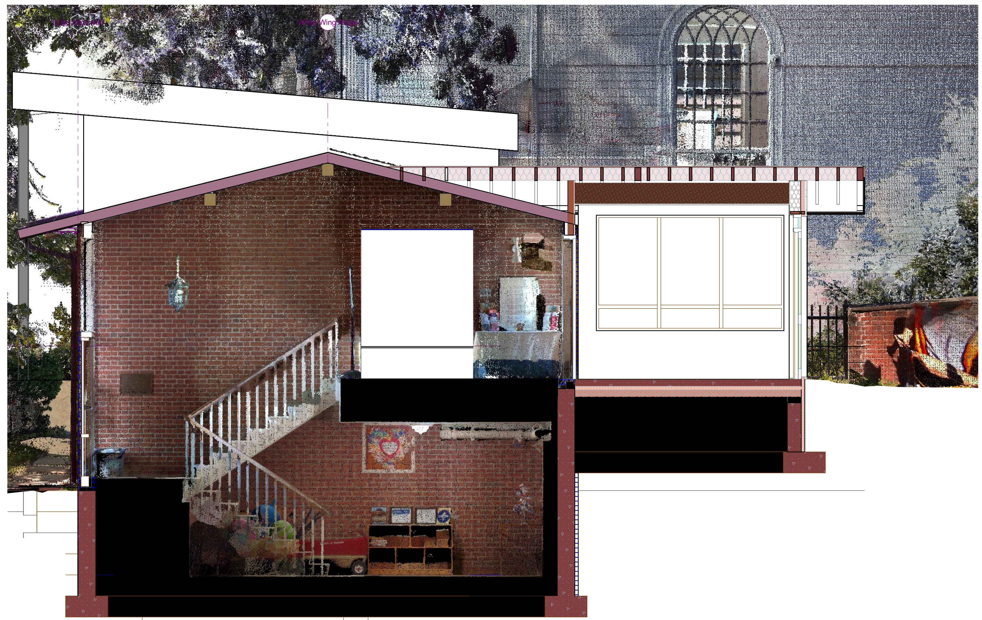
3 Section White Wing Stair WEST SCALE: 3/8" = 1'-0"
